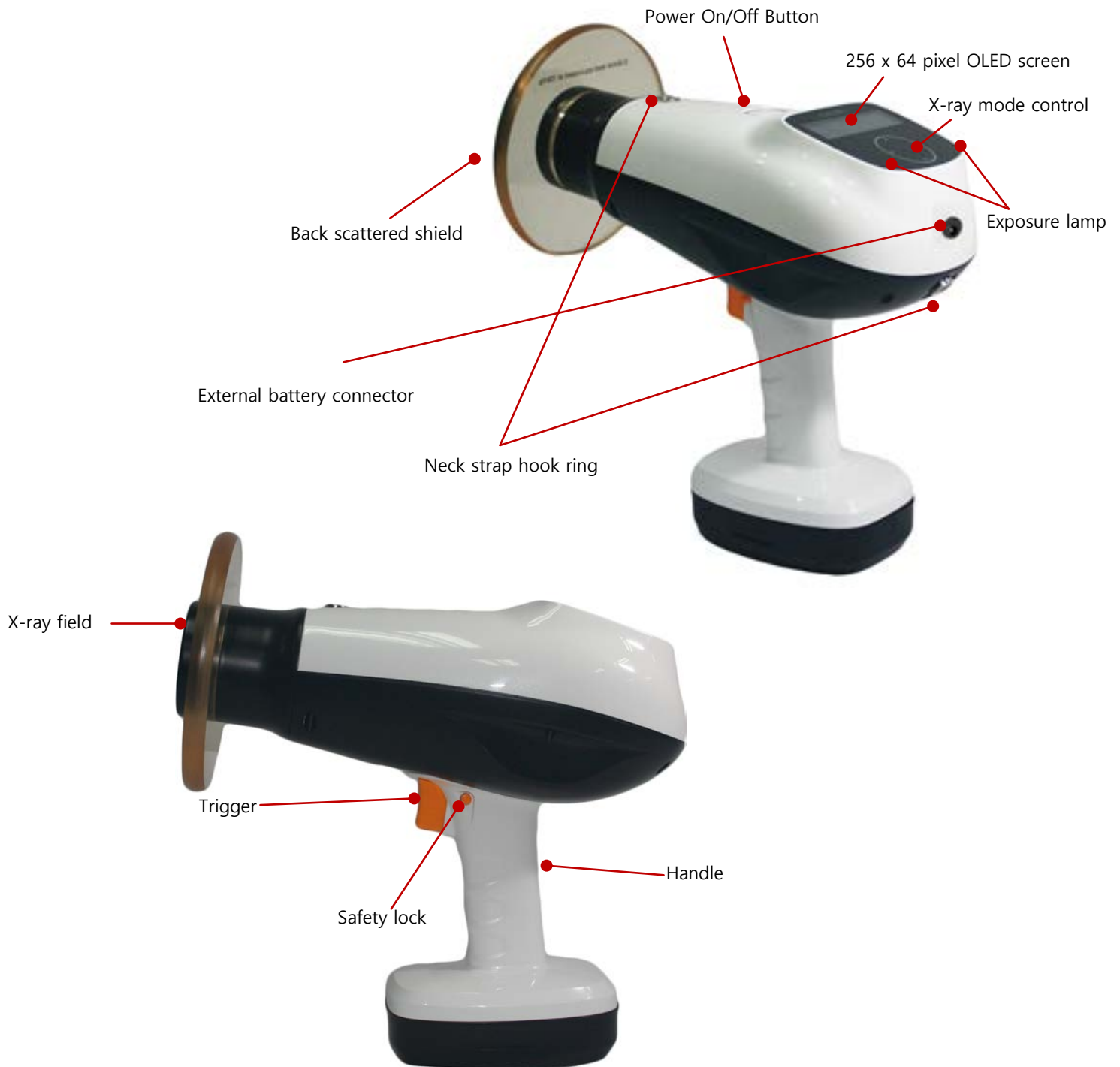
Figure 1.6 Each part name of main body (DX-7017/DX-7020)
