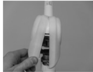
Step 4: Pry the LH cover up.
