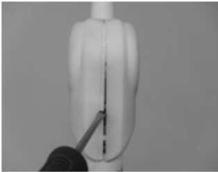
Step 3: Turn driver 90° to separate the covers.
