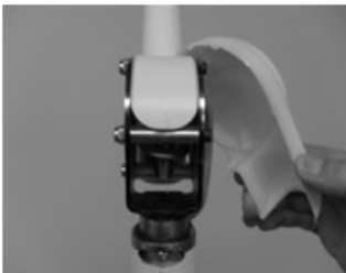
Step 7: Pry the RH cover forward.
