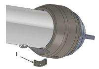
2.1.28 Remove the locking clip (1) from spring arm.
