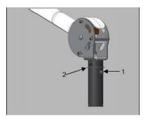
2.1.20 Remove the M4 allen screw and lock washer (1). Ensure the washer (2) stays in position.
